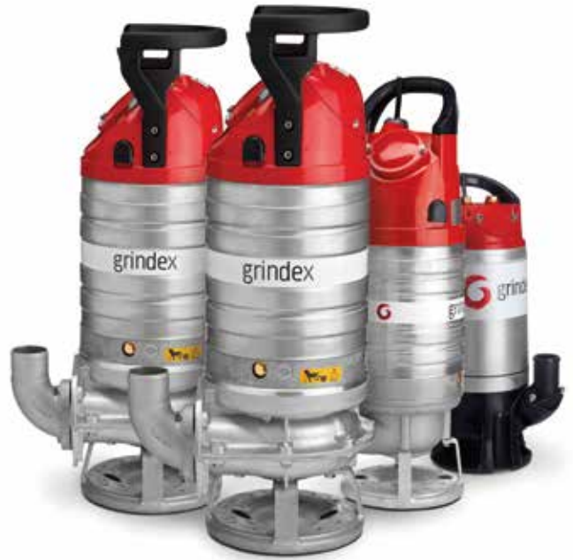
The sludge pumps are built to handle contaminated water, pH 5-8, and water containing relatively abrasive solids up to the size of 80 mm.
